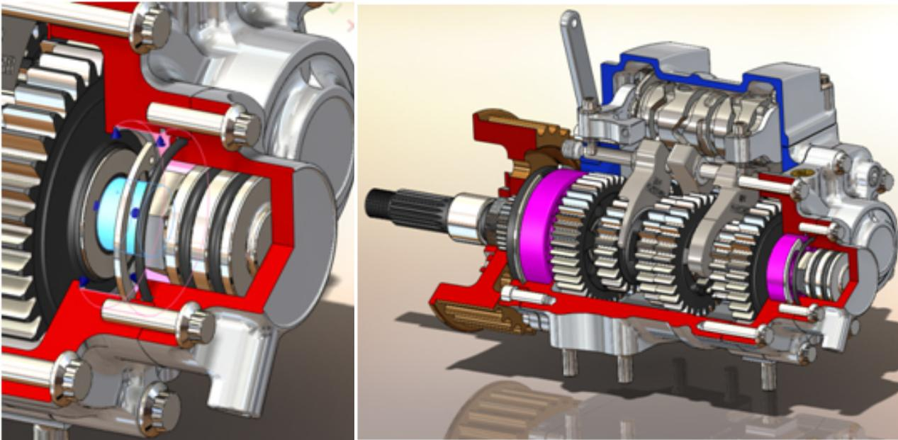
Figure 4. The gearbox bearings (pink) can be replaced by bearing connectors (blue) to accelerate the simulation solution.
