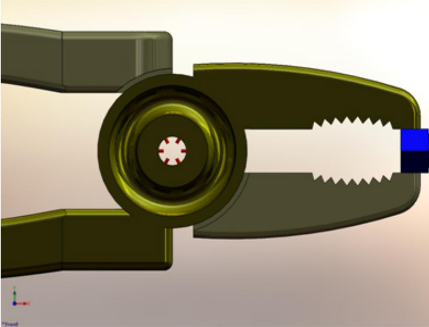
*The pin connector can simulate pins that rotate, slide back and forth, or both rotate and slide.*
