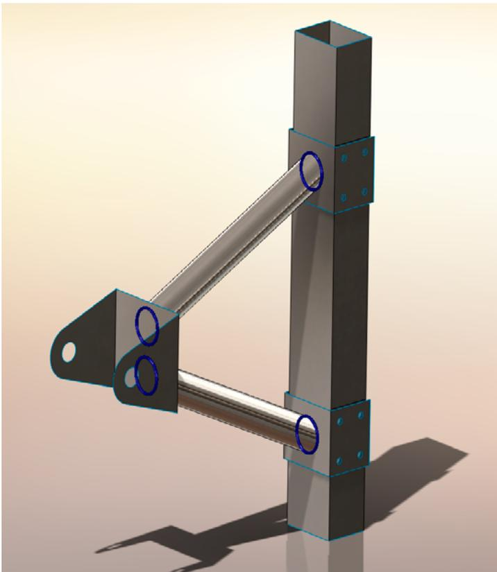
Figure 10. Edge welds (dark blue) join parts of a brace together
