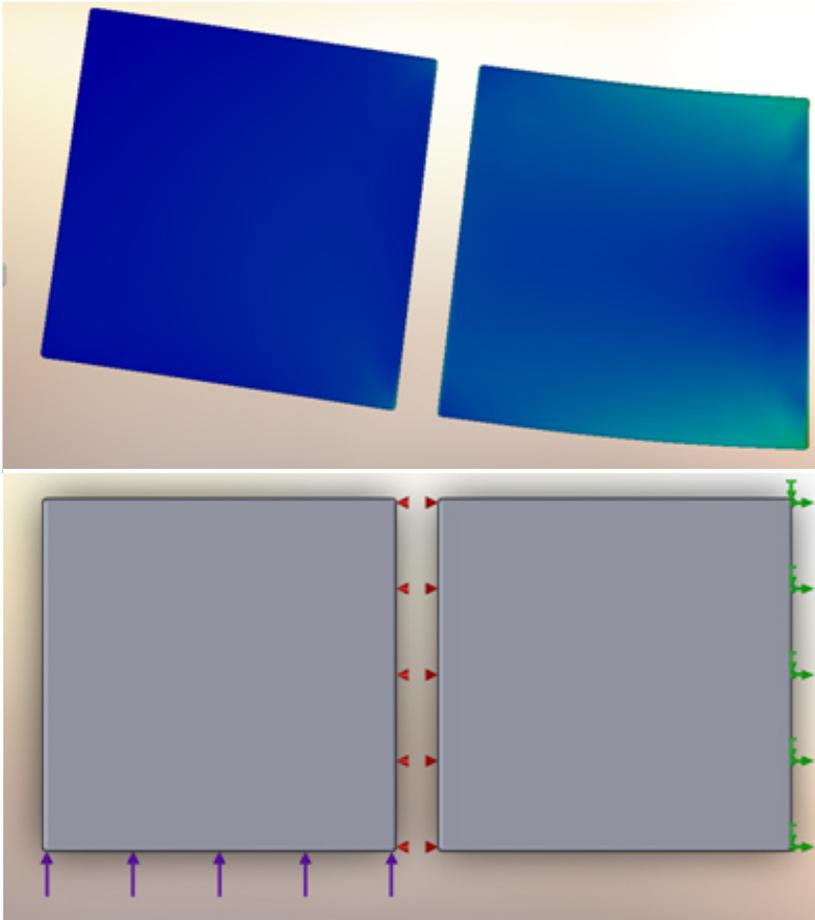
Figure 12. A rigid connector keeps the two middle surfaces fixed with respect to one another even after significant loading
