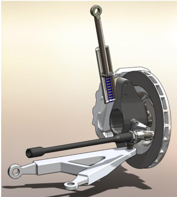
Figure 3. Section view of a piston with a spring-damper connector (in blue)
